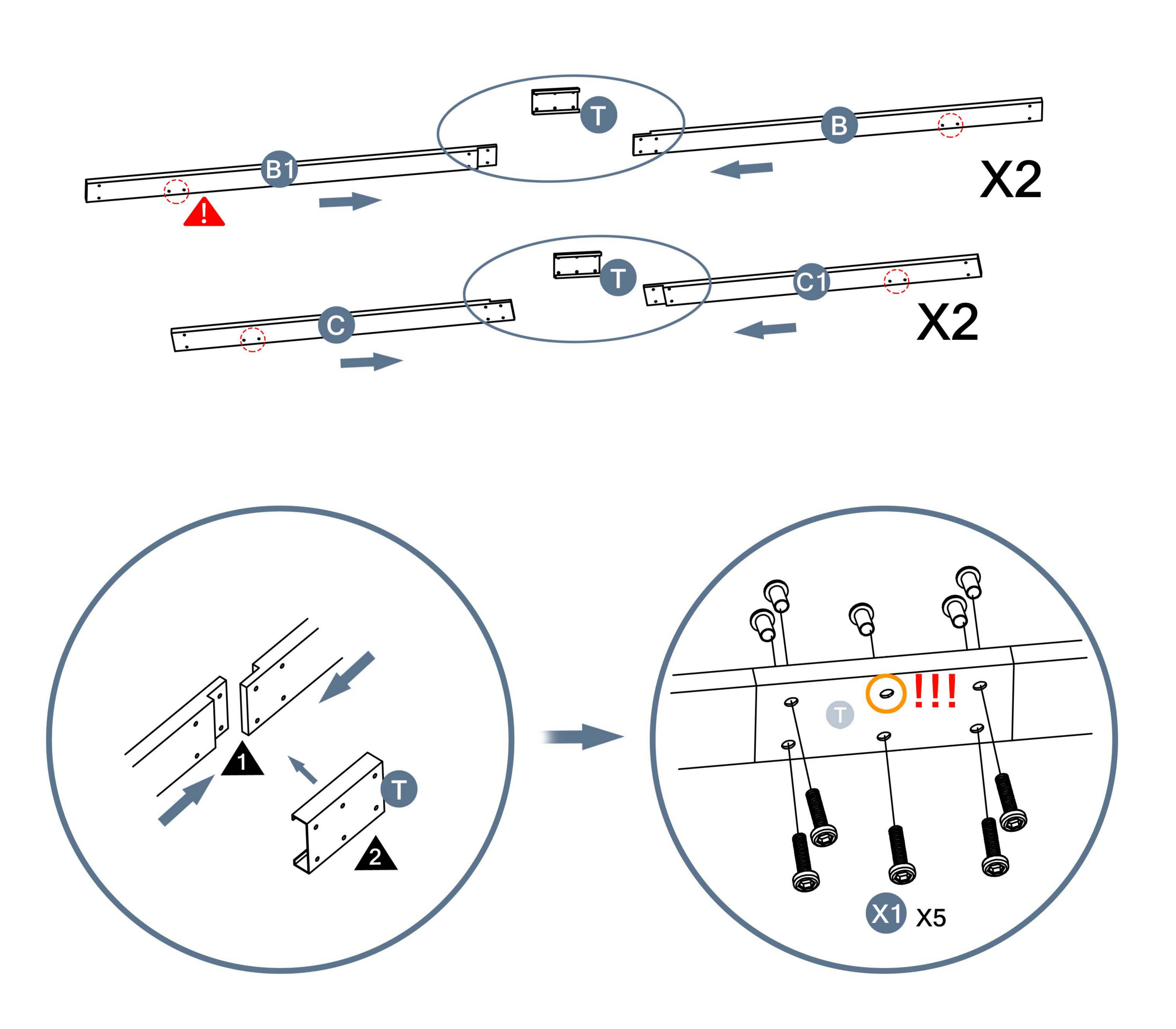
Be careful not to screw the screws at the yellow circle. Step 5 is screwing.
