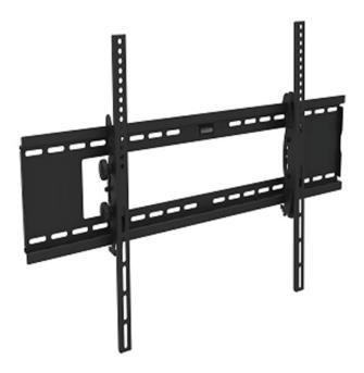
The wall mount WM-6090 supports 55" to 90" flatscreen TV's weighing up to 220 lbs. Vesa max 900 x 500mm. Tilt range is -15 to +15 degrees. Generic wall mounts are not manufactured by us and are provided for your convenience. We tested for strength and compatibility with our accessories.
