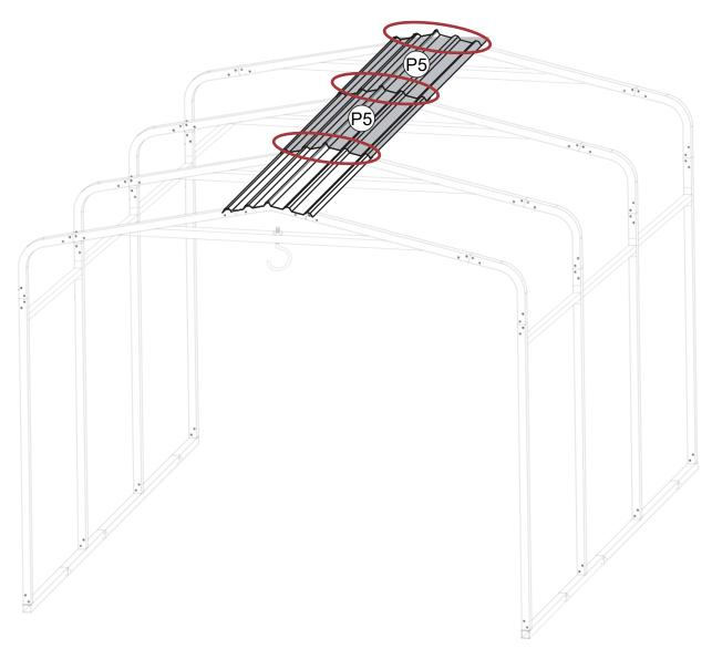
Apply a layer of waterproof tape to the outside of the seams of the two layers of tin, which can effectively prevent leakage of the carport
