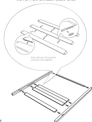
Ensure best face is forward and insert rails into legs.
