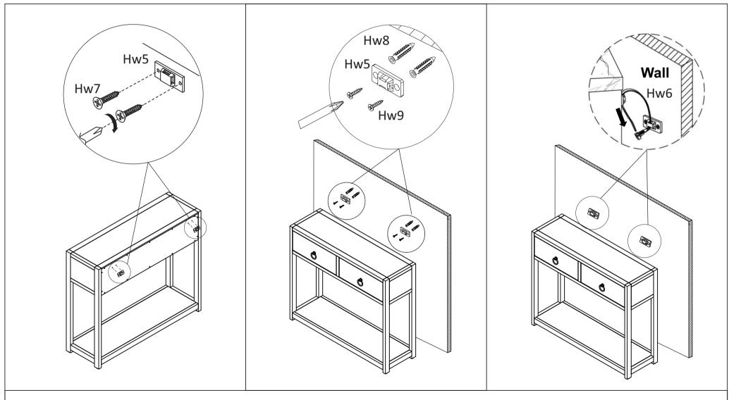
Step 3: PLEASE NOTE: To help prevent the possible of tip-over, install the tip-over restraint provided.
