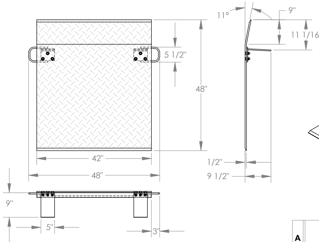
NOTE: BEND OR CROWN IS 11° AND LOCATED 9" FROM EDGE OF DOCKPLATE
