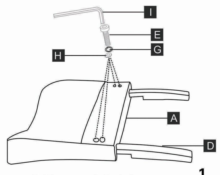
Put the screws in the holes, tight the screws, but not too tight, 100% is ok.
