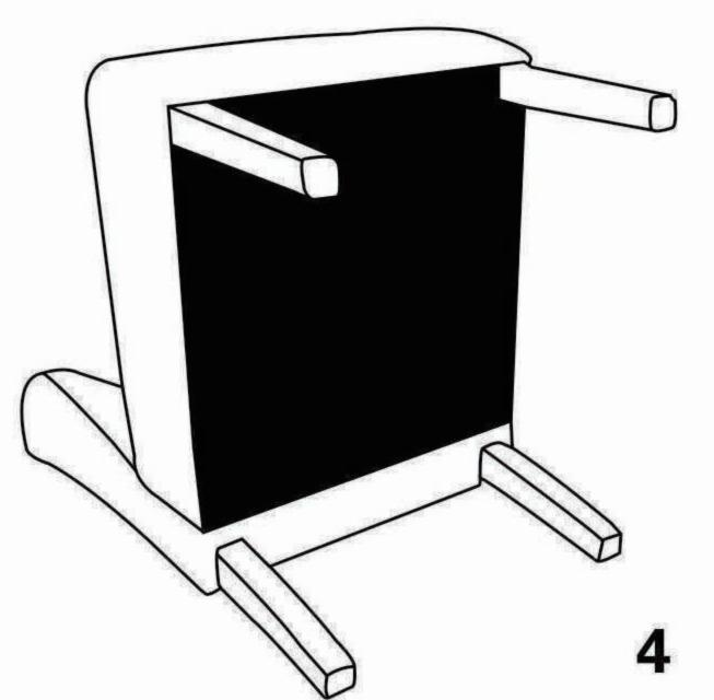
Stand the chair upright&ensure it is level before tightening all screws, Then tight all the screws to 100% Then Stick the black part on the seat
