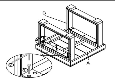
Attach the remaining Leg Frame(B) to the Table Top(A) using Bolts( $\widehat{1}$ ) and the Allen Key( $\widehat{2}$ ).
