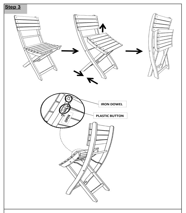
**To close,** pull the Seat up and fold Iron Leg Frame as indicated by the arrows, by hand, until the Chair folds shut
