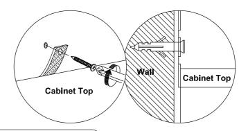
NOTE: Wall fixings are not supplied with this product as different wall materials require different types of fixing devices (such as Rawl plugs on brick work). You must use fixing devices suitable for the type of wall you intend to mount this product to. Please ensure that the head of any screw used as a diameter greater that the diameter of the mounting hole on the bracket and that the fixing is safe and secure before use.
