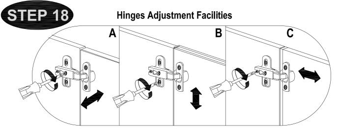
A.Lateral adjustment by screw adjusting
