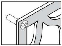
• Using spacers to set the panel off the wall or fence will create a more 3-dimensional installation with shadow effects. Backlighting can be used to further enhance this effect. Holes in the panel must be 3/16" larger than the screws.
