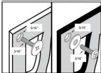
Using the MATRIX Screen Mounting Kit or screws and washers – holes in the panel must be larger than the screws by 3/16" to allow for expansion and contraction with changes in temperature. Do not overtighten screws to allow the panel to expand and contract.
