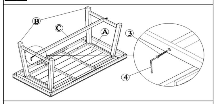
Insert the tenons on the Leg Support Bar(C) into the mortises of the Leg Panels(B). Attach Leg Support Bar(C) to Leg Panels(B) using Screws(3) with Allen Wrench(4) as shown above.
