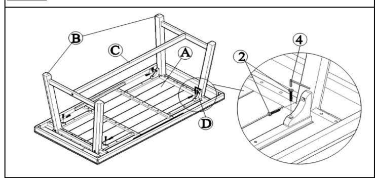
Align the Corner Blocks(D) to the Table Top(A) and Leg Panels(B) and attach using Screws((2)) with Allen Wrench((4)) as shown above.
