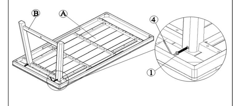
Attach Leg Panel(B) to Table Top(A) using Bolts(1) with Allen Wrench(4) as shown above.
