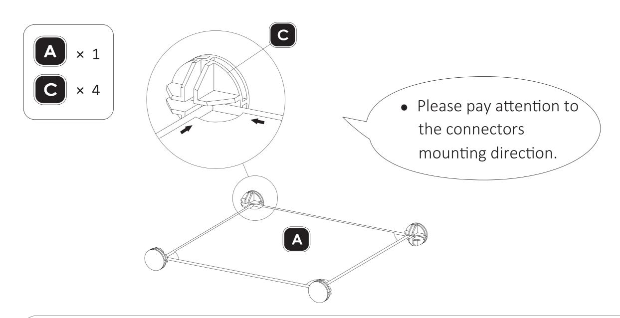
Before next step, please make sure assemble the shelf corner to the end of the connector hole.
