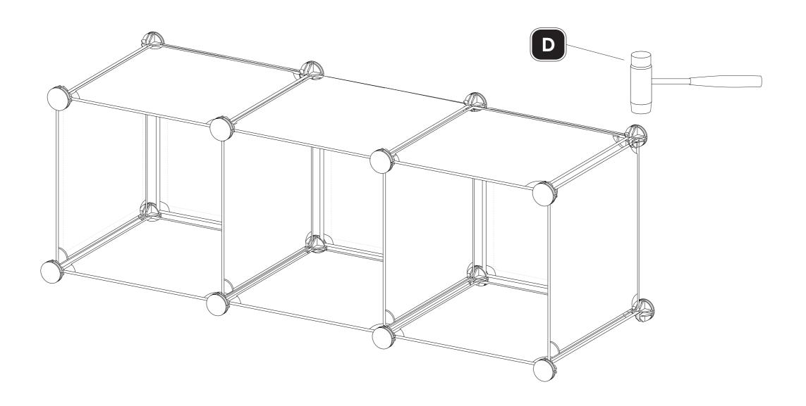
To tighten the connections between the every part, please knock down each connector with the hammer to secure the shelf corner are assembling to the end of the connector hole.
