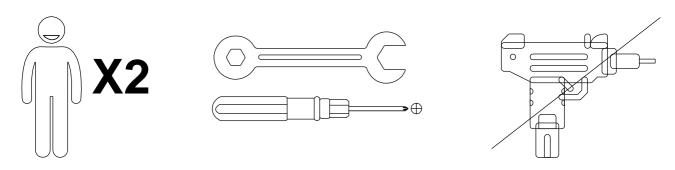
We recommend using hand tools for assembly. If an electric screwdriver is used, reduce power and torque to avoid damage to the product.
