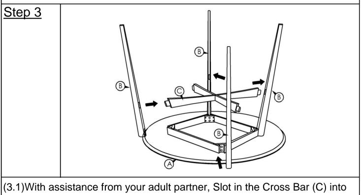
the mounting position of Table Leg (B) as shown.
