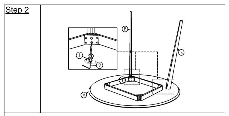
Place the Table top (A) on a soft surface to avoid any scratches or damages to the product and place the Table Leg (B) onto the of table top corner block with your adult partner.
