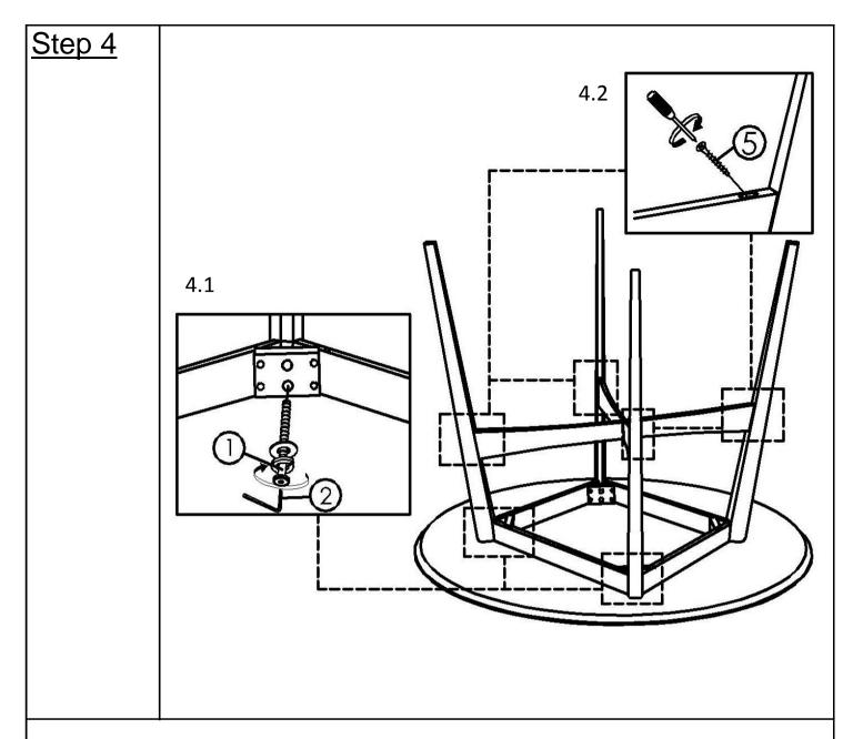
4.1 Repeat step 2, Fix the Table Leg (B) with JCBB Bolt ① + Spring Washer
