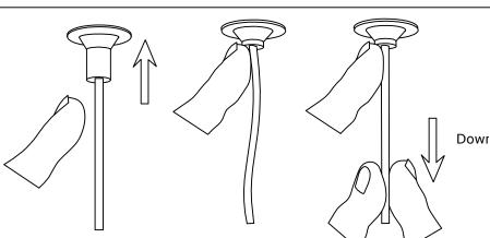
1.simply push up on the cable to raise the height of the fixture
