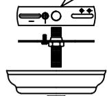
1. Fasten the light fixture by using the collar loop.
