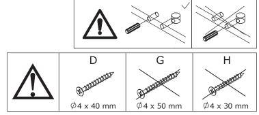
Secure part 24 to parts 16, 22, 22, 19, 23 using dowels (C) and screws (D).
