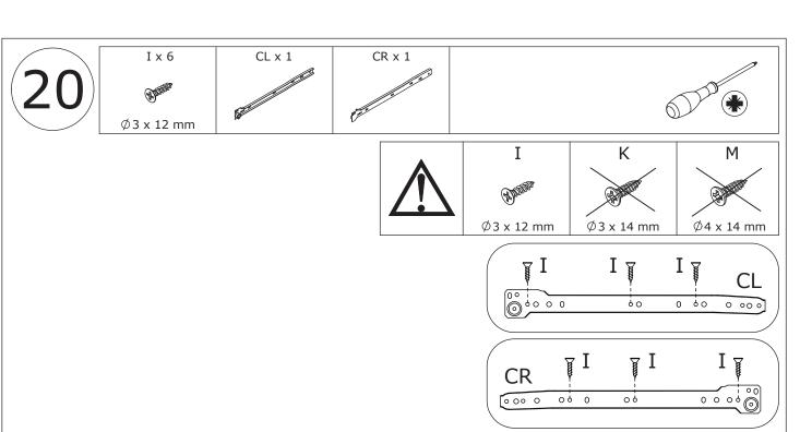
Use screws (I) to fix the guide rail (CL) to part 18 and screws (I) to fix the guide rail (CR) to part 21.
