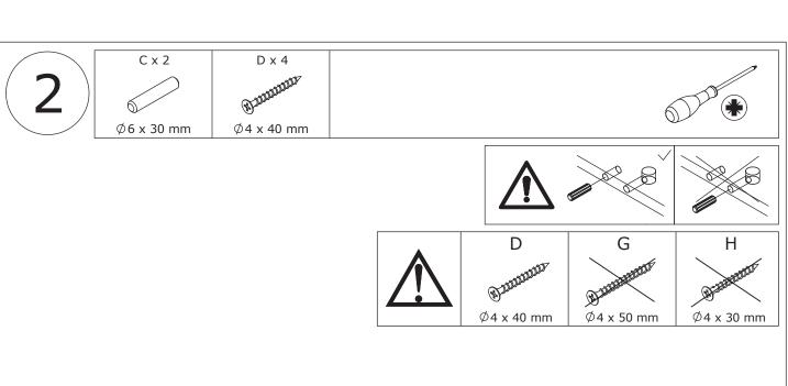
Attach part 1 to part 2 using dowel (C) and screws (D).
