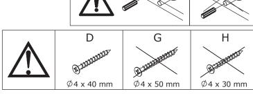
Secure part 15 to part 14 using dowels (C) and screws (D).
