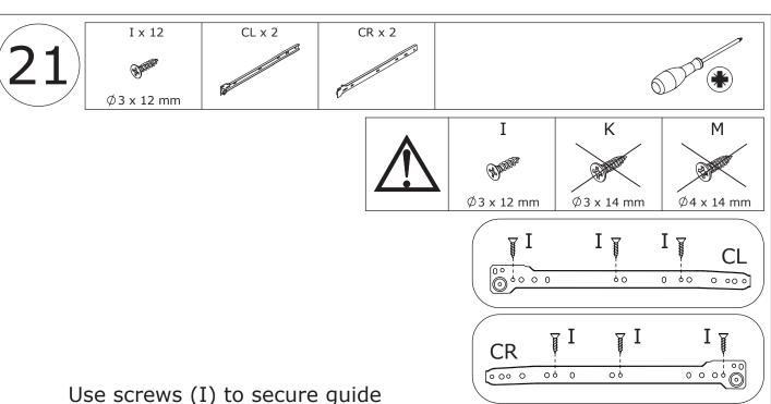
Use screws (I) to secure guide rails (CL) to part 22, use screws (I) to secure guide rails (CR) to part 22.
