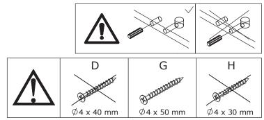
Secure part 11 to part 10 using dowels (C) and screws (G).
