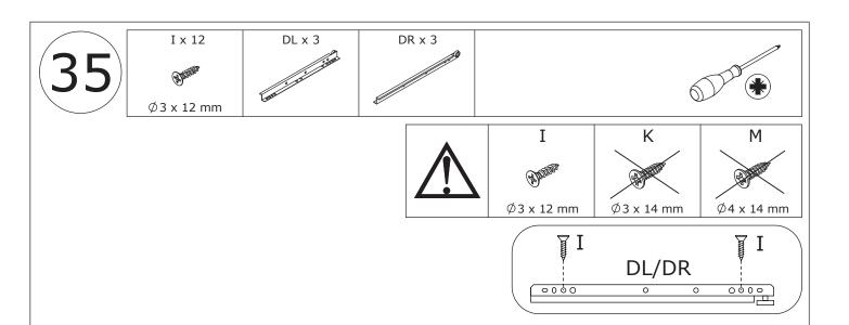
Secure the guide rail (CR) to part 32 using screws (I) and the guide rail (CL) to part 30 using screws (I).
