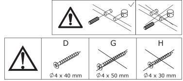
Use dowels (C) and screws (D) to attach part 24 to parts 25, 26, 25, 26.
