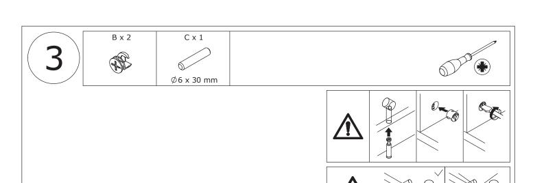
Attach part 3 to part 2 using the dowel (C) and tighten the cam lock by turning it clockwise using the cam lock (B).
