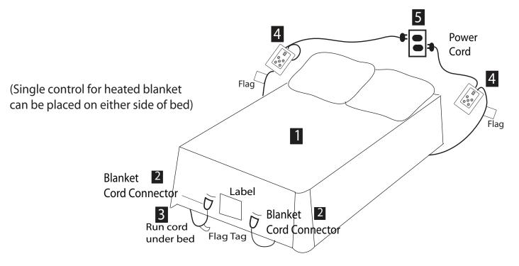
5. Plug the power cords into a 110-12 volt wall outlet. CAUTION: Do not use with generator power or plug into an extension cord or power strip.
