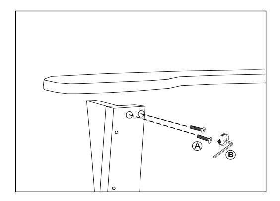
IMPORTANT: DO NOT TIGHTEN BOLTS COMPLETELY UNTIL ALL BOLTS ARE COMPLETELY LINED UP AND INSERTED INTO HOLES.
