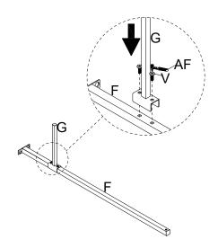
Attach the Center Rail - Front / Rear (F) to the Headboard (A) and the Footboard (B), insert the Bolt (V), turn the Ratchet Tool (AF) to tighten them. Then attach the Center Rail - Front / Rear (F) to the Center Support Bar (C), insert the Bolt (W), turn the Ratchet Tool (AF) to tighten them.
