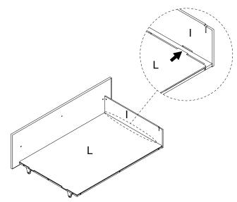
Insert another Drawer Side Board (I) to the Drawer Bottom Board (L) first, and attach the Drawer Side Board (I) to the Drawer Bottom Frame (K), then insert the Bolt (X) and Washer (AD), turn the Ratchet Tool (AF) to
