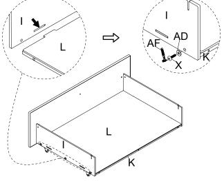
Attach the Drawer Back Board (J) to the Drawer Bottom Frame (K), insert the Bolt (X) and Washer (AD), turn the Ratchet Tool (AF) to tighten them. Attach the Drawer Board Connector (Q) to the assembled drawer, insert them into correct places.
