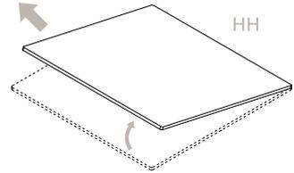
Rotate the panel when inserting.
