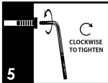
5 Make sure all parts are properly aligned, then use the appropriate hand tool to completely tighten the bolts or screws. Do not use power tools and do not overtighten.
