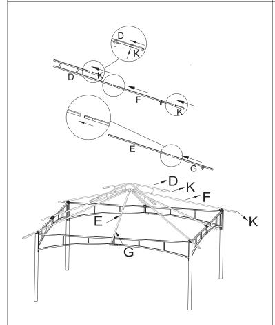
Step 3:Insert the small head of Part F to the long side of Part D directly and insert one Part K to the other head of Part F.Then insert one Part K to the short side of Part D.Insert the small head of Part G to Part E.
