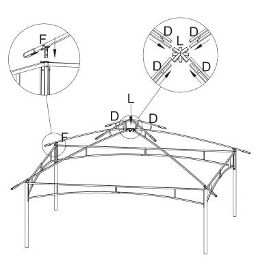
Step 4:Insert four Part F to the four corners of the frame (the top of Part A) . Then insert the other side(the bottom side of Part D) to Part L. 4
