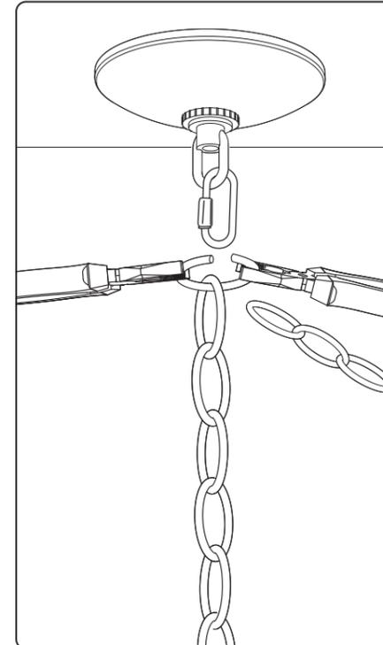
3. Connect the Quick Chain Link to the Chain Holder. Determine the height you want to hang the fixture down from the ceiling. Use a pair of pliers to twist open the chain link end and remove the unwanted portion of chain. Connect the wanted chain to the Quick Chain Link. Twist to close both opened chain links.
