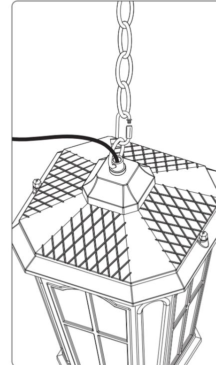
4. Connect the fixture and the chain with the Quick Chain Link.
