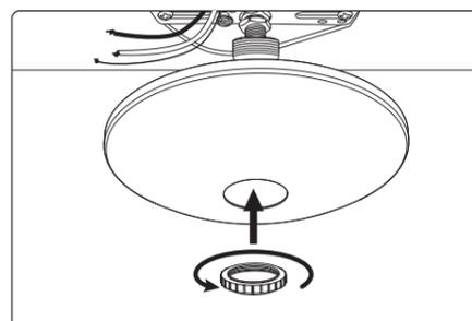
2. Attach the Canopy to the ceiling using the Screw Collar.
