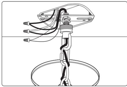
6. Make the following spliced wire connections using wire nuts:
