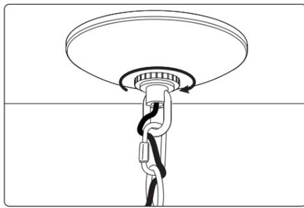
7. Put the Canopy back up against the ceiling and lock it in place using the Collar.
