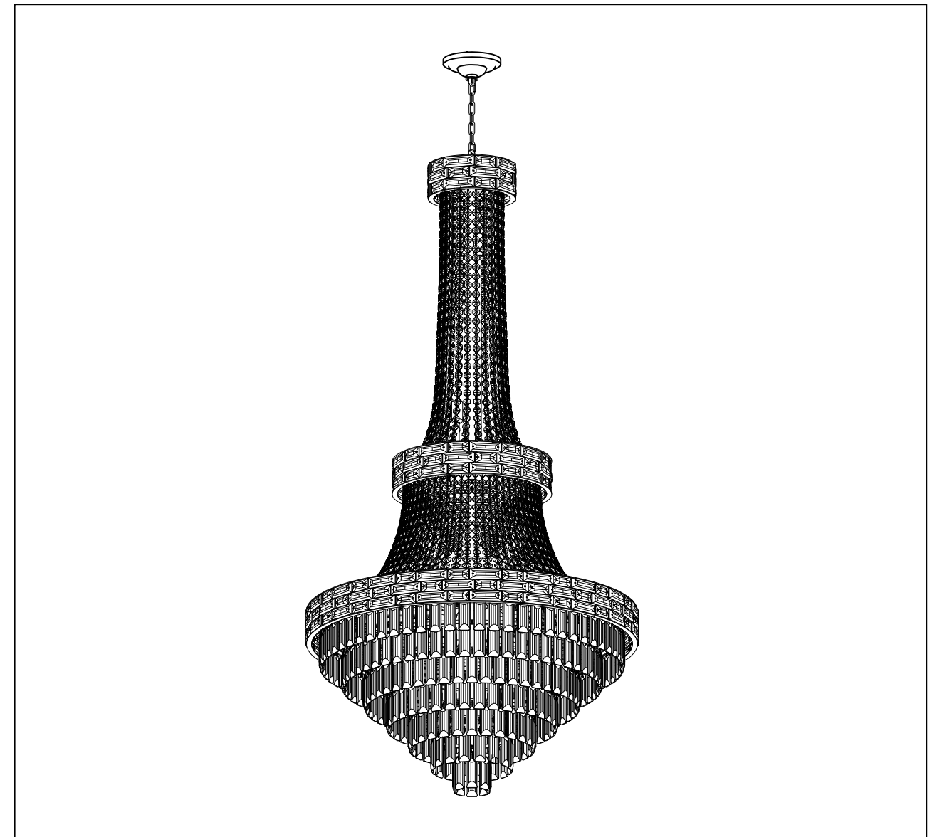
2.Hang all the crystals as shown(Please hang crystals in order from bottom to top)
