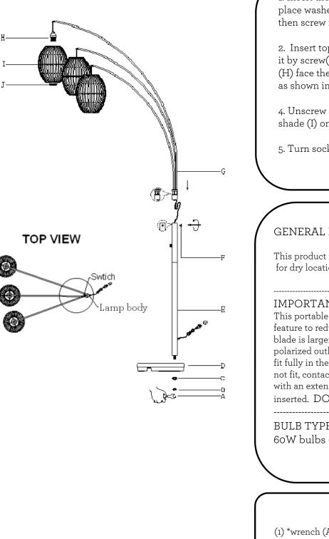
1. Insert the tube (E) through base (D), and place washer (C) and nuts (B) under base (D), then screw nuts (B) by wrench (A) until tight.
