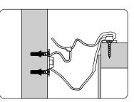
The screw and plug supplied can be used with most solid and hollow walls. For solidwood use the screw without plug.
