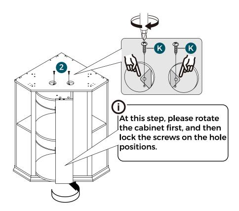
Caution: Inappropriate installation of screwswill cause damages to the product!
