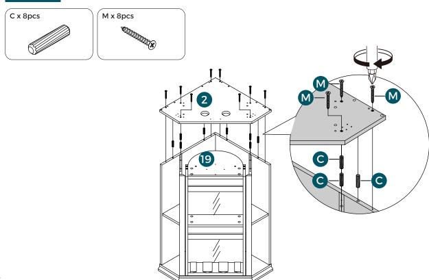
Caution: Inappropriate installation of screwswill cause damages to the product!
