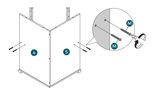
Caution: Inappropriate installation of screwswill cause damages to the product!
