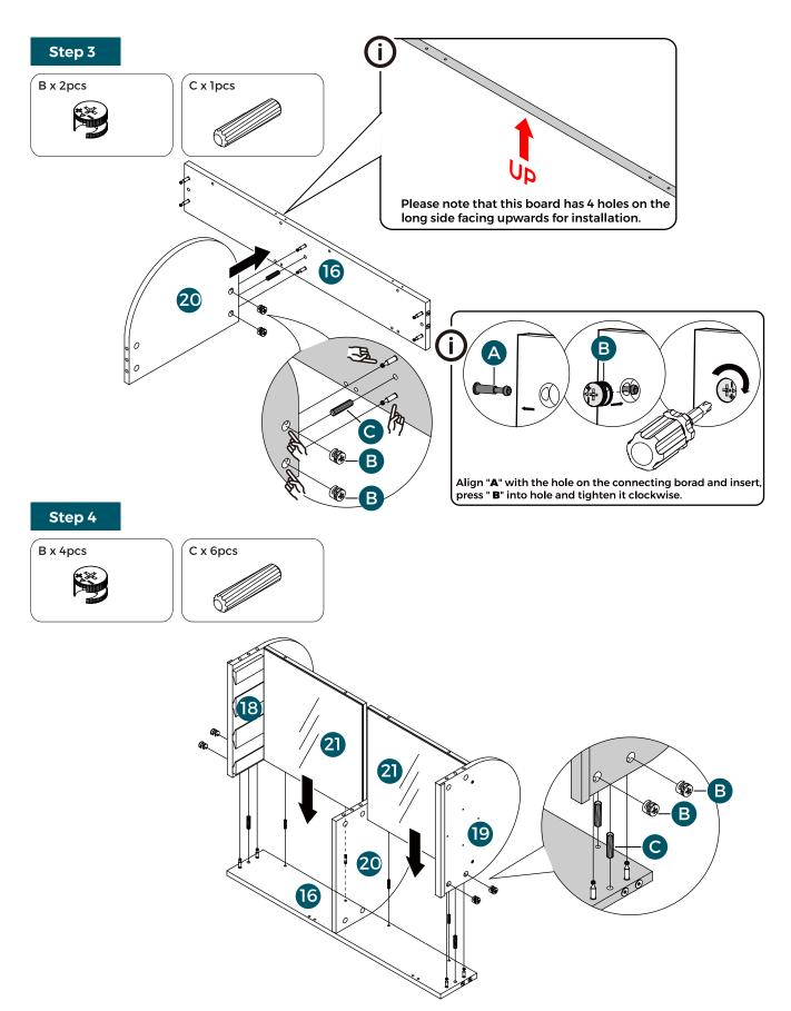
Caution: Inappropriate installation of screwswill cause damages to the product!
