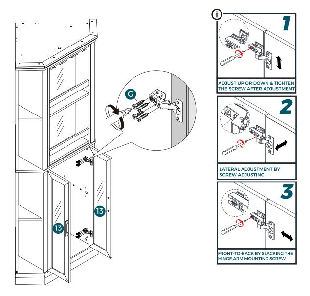
Caution: Inappropriate installation of screwswill cause damages to the product!
