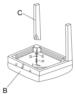
Put chair back (A) on a smooth flat surface, attached the seat (B) the chair back (A) use the bolt (F), lock washer (D), flat washer (E) in both of hole of seat (B) and chair back (A), turn the allen wrench (I) in bolt (F). But not too tight.
