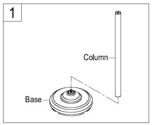
1. Put the base in a level space on ground. Thread one end of column into base tightly with clockwise direction.
