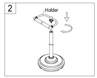
2. Install paper holder into another end of the column tightly with clockwise direction.
