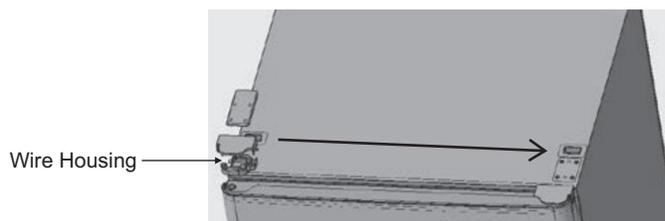
4. Remove the plastic wire housing piece.
