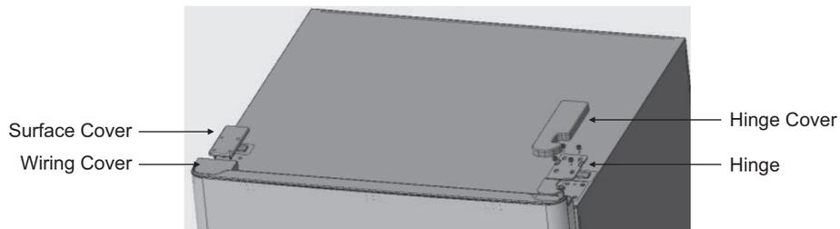
1. From the left top of the unit, remove the top cover that covers the wiring (wiring cover).
