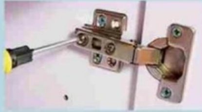
The gap between the door panel and the side panel is too large
