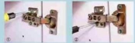
The door panels are uneven in height
