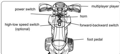
All switches are on the dashboard of the car. For high-low speed switch is option, only customer choose this dispose the car will have.
