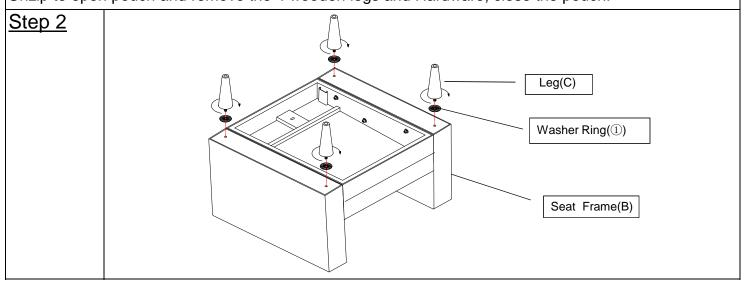
Install the Legs(C) into the bottom of the Seat Frame(B) by placing a Washer Ring(1) onto the threaded stem of the Legs.
