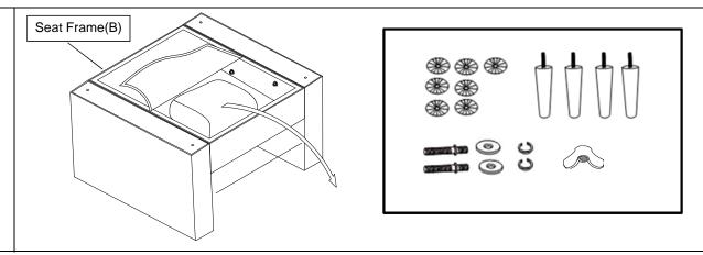
Position the Seat Frame(B) on its back, as shown.
