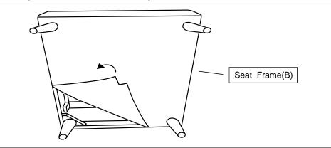
Cover the bottom of the Seat Frame (B) with the non-woven fabric. Smooth down the Magic Tape on all four sides of the Seat by hand.
