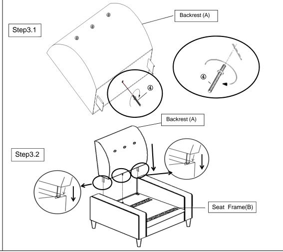
Step 3.1 Screw-in the short end of Screw Arbor(4) into Backrest(A), by hand, turning clockwise as shown.
