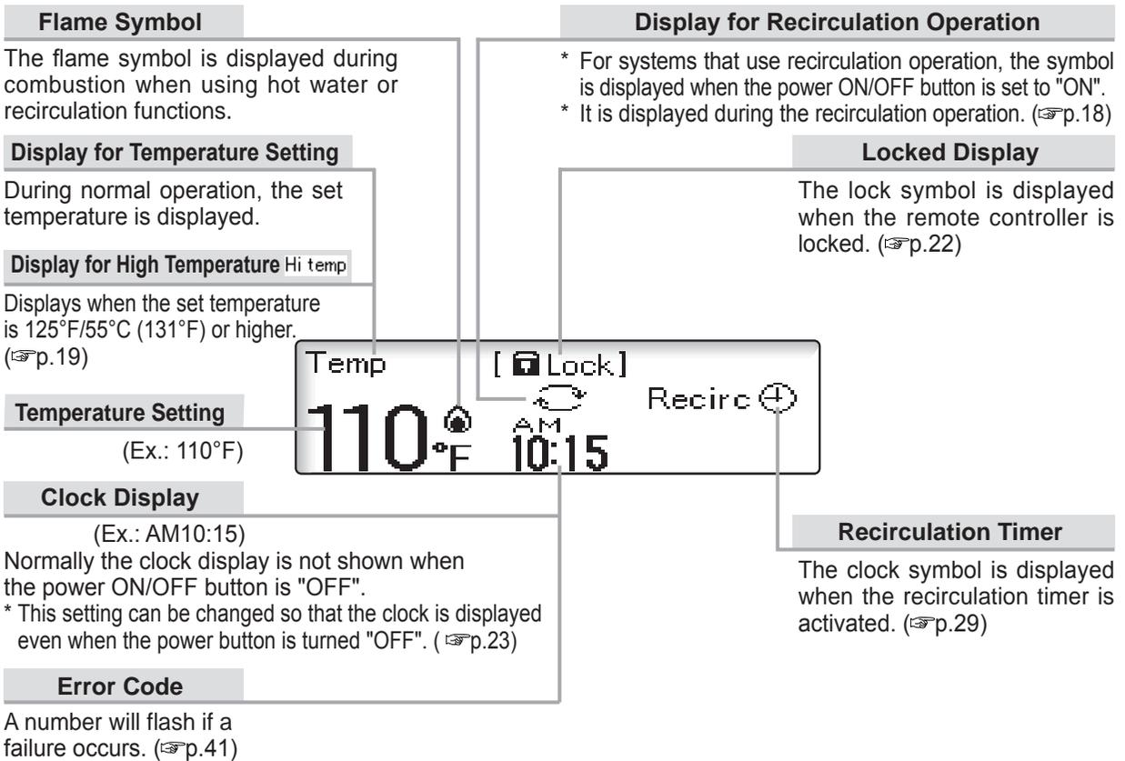
Note: As shipped from the factory, the remote controller is set to display in °F and gallons.
