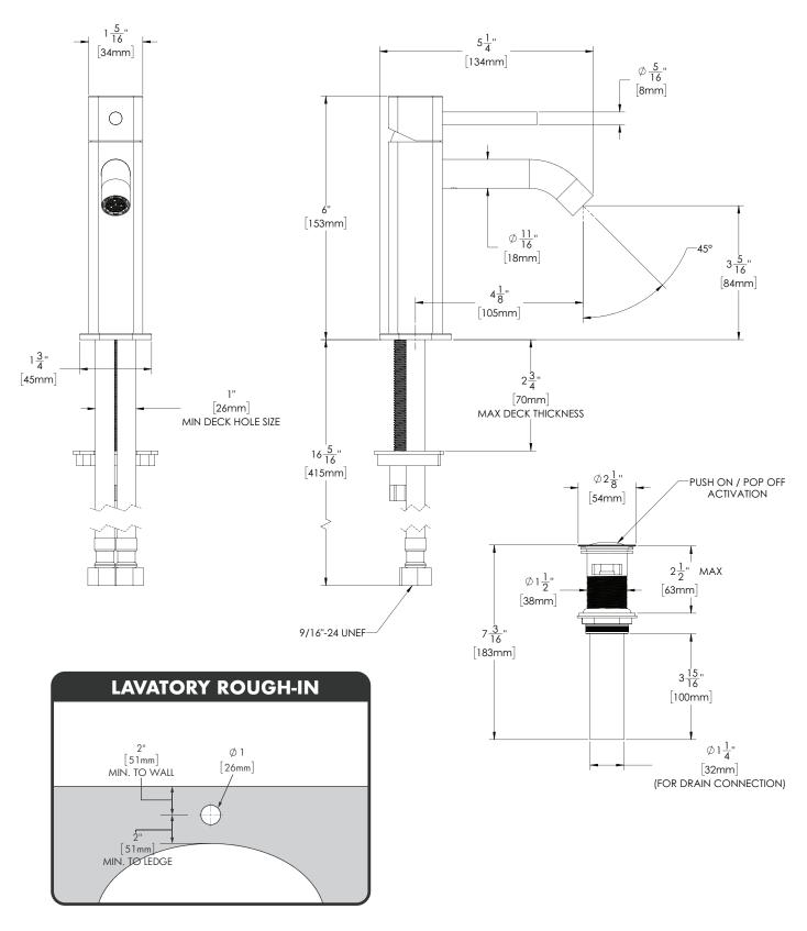
1. All dimensions are in inches (millimeters) unless otherwise specified and are subject to change without notice. 2. Contractor to supply necessary inlet connections.
