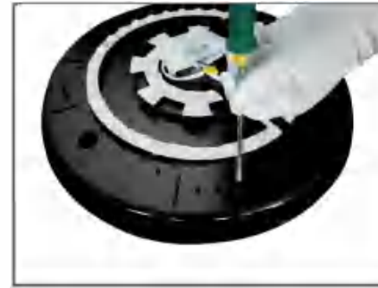
Step 4. Remove the main engine chassis screws.
