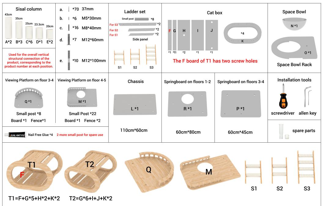
For the convenience of installation, it is recommended to assemble T1, T2, Q, M, as well as S1, S2, S3 in advance, and then install the overall part from bottom to top.
