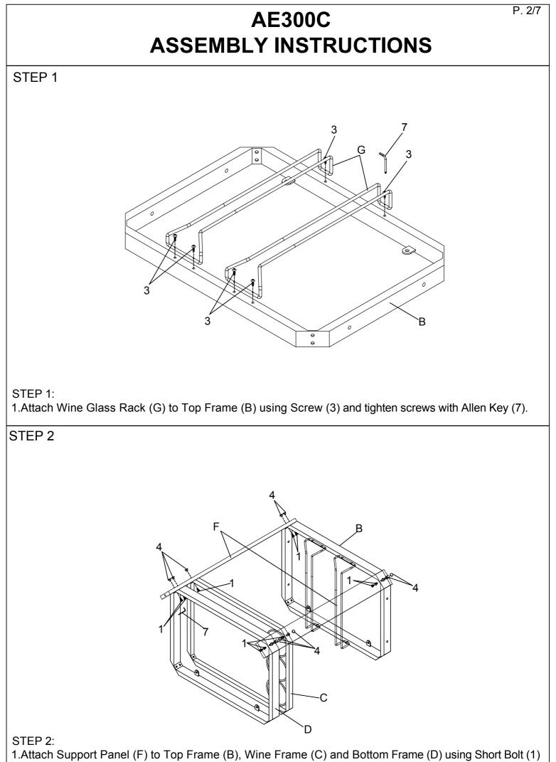
, Nut (4) and tighten bolts with Allen Key (7).
