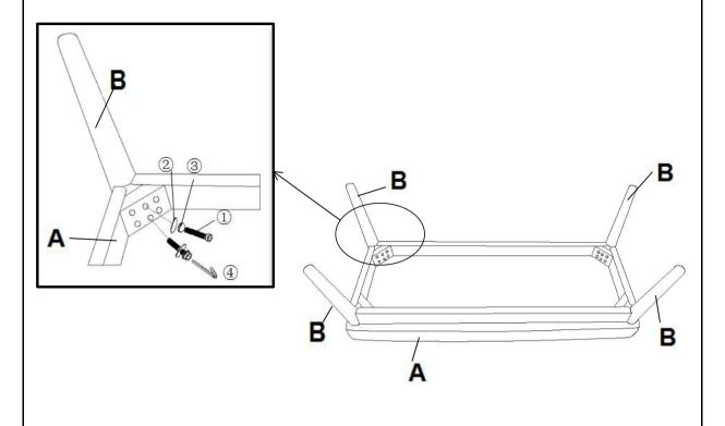
Insert one Wooden Leg(B) into the mounting position of the Ottoman(A).
