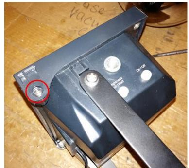
Loosen the screws on the side of the faceplate. There is one screw on each side.
