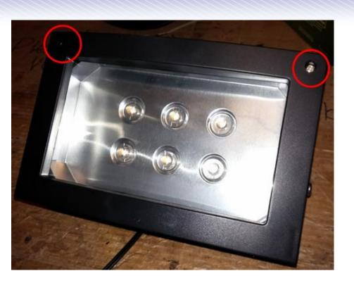
Remove the circled screws from the nuts.
