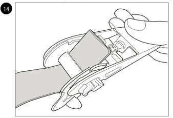
Raise and lower the handle two or three times to wind the strap onto the spindle (fig. 15).
