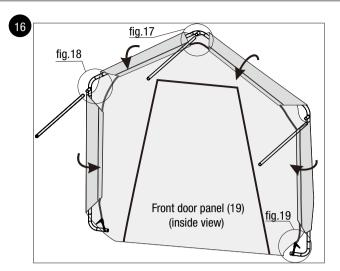
• Locate the top part of the front door panel (19) near the 3-way peak connector (11), disconnect the shoulder cross rail (4) from the 3-way peak connector (11), and pull the strap onto the connector (11). Then re-insert the cross rail (4) to its proper position (fig. 17).
