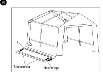
• Stretch the roof tarp (18) over the shed frame and make sure it is centered on the frame (fig. 21). Use a ladder if necessary.
