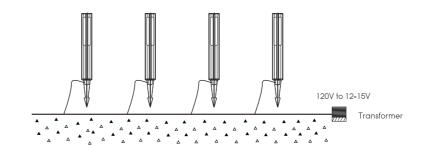
Step 6: Use a shovel to loosen the ground or soften it with water, then place the fixtures into the ground and the wire inside the dug ditch and cover it with the surrounding dirt. The transformer can now be plugged in.
