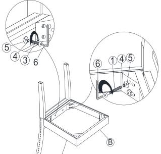
Attach front legs (C) to the seat frame. Use bolts (2), washers (4) and (5). Tighten with Allen Key (6). Attach bottom removed on the step 1 on seat frame.
