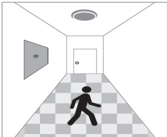
With sufficient daylight, even when motion is detected, light remains OFF.
