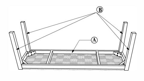
Step 2: use hex wrenches to connect the legs with seat part by bolt and washer.
