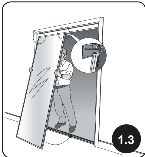
1.3 Tilt a door panel, insert the top rollers in the rear « J » channel of the top track..
