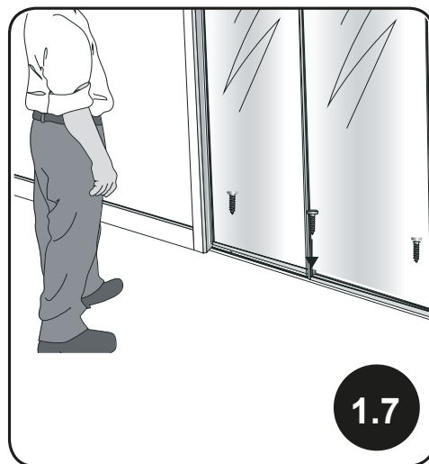
1.7 Once equalized, fix the bottom track with the short screws.
