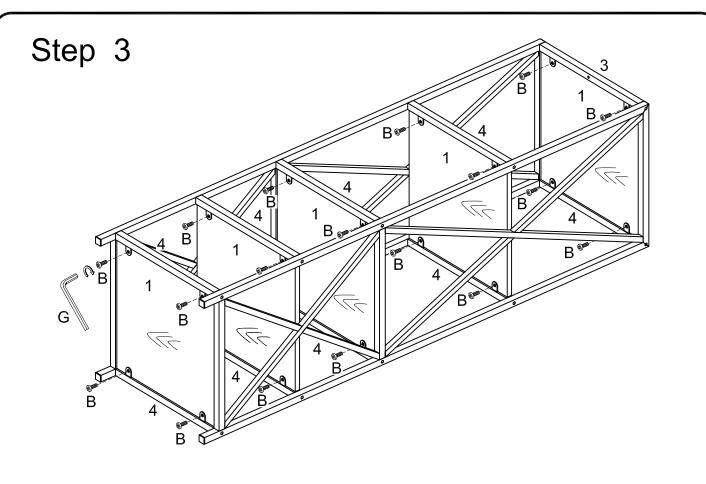
Use Wrench (G), Bolt (B) to secure the shelf (1) to the Support Bar (3, 4).
