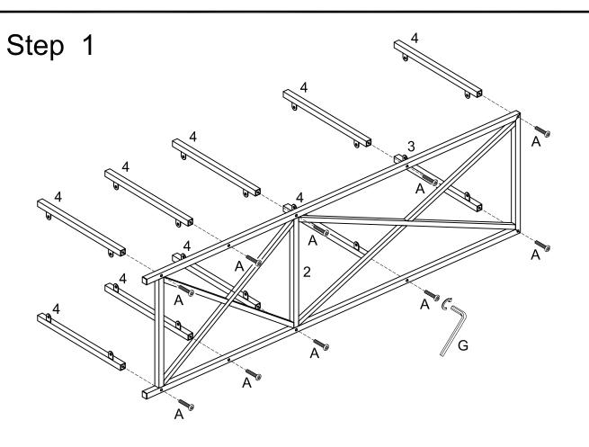
Use Wrench (G), Bolt (A) to secure the Support Bar (3, 4) to the Side Frame (2).
