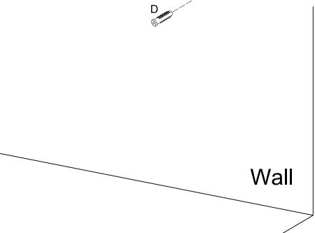
Insert the Wall Anchor (D) to the Wall.
