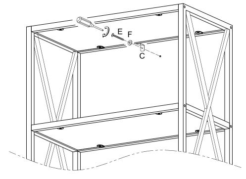
Secure the Screw (E), Washer (F) and L Shape Bracket (C) against the Wall as per diagram.
