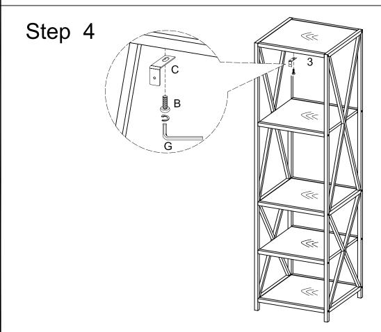
Use Wrench (G), Bolt (B) to secure the L Shape Bracket (C) to the Support Bar (3).
