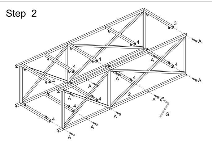
Use Wrench (G), Bolt (A) to secure the Support Bar (3, 4) to the Side Frame (2).
