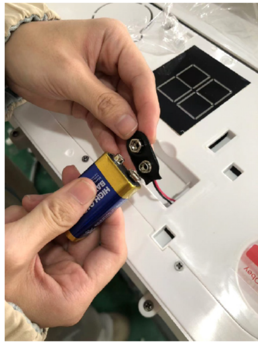
Step 2 Connect the battery.
