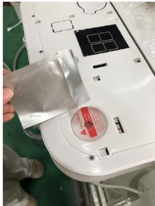
Step 2 Peel off the protective film on the aromatherapy tablet slot.
