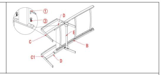
As shown above, install part (E) to part (C, C1) using the Bolts(③) with Allen Wrench (①). **Do not fully tighten the Bolts.**
