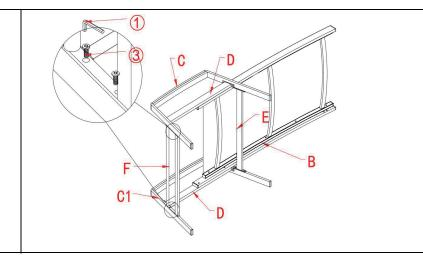
As shown above, install part (F) to part (C, C1), using the Bolts(③) with Allen Wrench (①). **Do not fully tighten the Bolts.**
