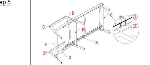
As shown above, install part (G) to part (B), using the Bolts(③) with Allen Wrench (①). **Do not fully tighten the Bolts**.
