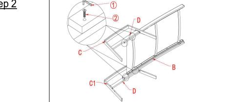
As shown above, install part (C, C1, D) to part (B) using the Bolts(2) with Allen Wrench (1). Do not fully tighten the Bolts.
