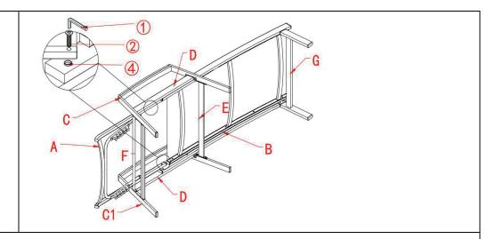
As shown above, install part (A) to part (B), using the Bolts (②) and Washer (④) with the Allen wrench (①).
