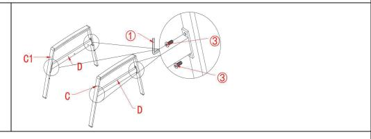
Open the carton and place all parts on a clean, non-marring surface. As shown above, install part (D) to part (C, C1), use the Allen Wrench (1) to tighten the Bolts (3). Fully Tighten the bolts.
